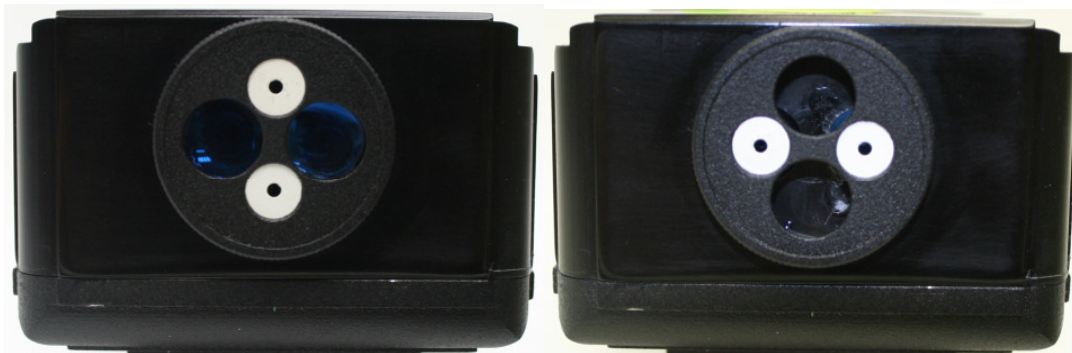
FIG.4.1. DIAPHRAGM POSITIONS. A) MEASUREMENT, B) ALIGNMENT
