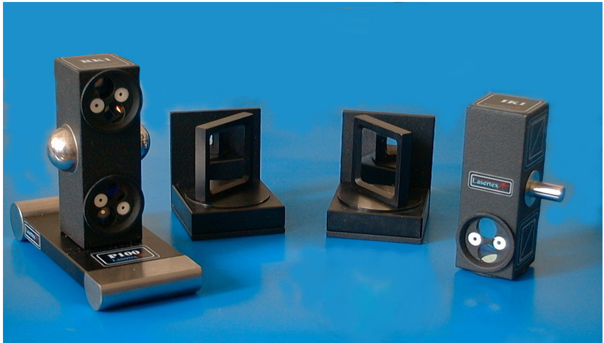
FIG.8.2. THE ELEMENT SET FOR THE FLATNESS MEASUREMENTS (IK1, RK1 ON P100 BASE AND BB2)
