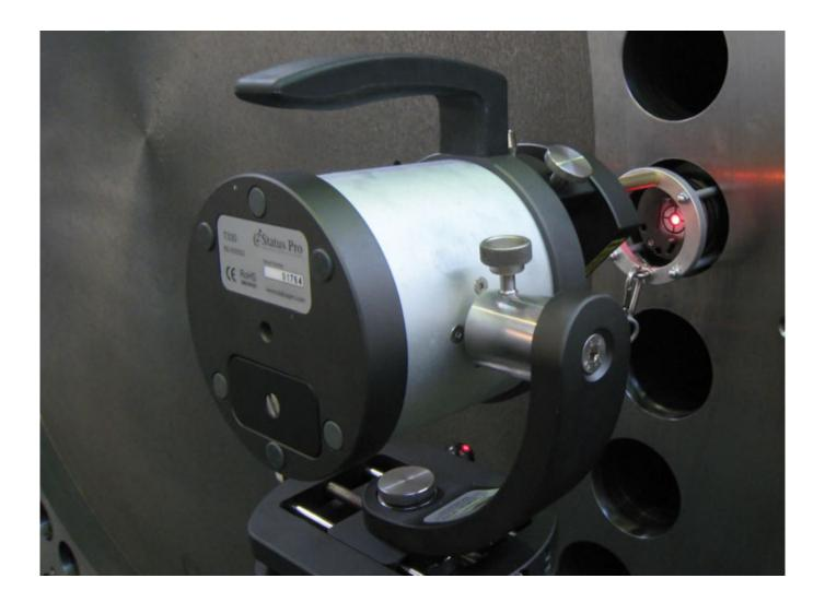
The measurement of deep hole drilling is always a special task, where besides the linearity, the circularity, the perpendicularity and the parallelism could be of importance.
