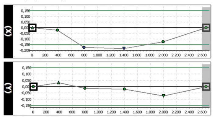
The first and the last point are set to zero. By doing this it is possible to analyse the deviations of the points between them.
