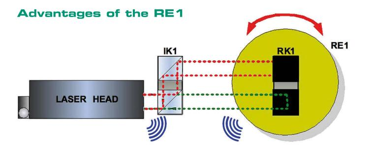
The RE1 Rotary Calibration Kit is capable of carrying highly reproducible and accurate measurements using a combination of "Gleason Toothing" and supplied optics.
