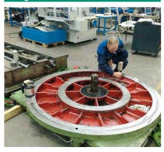
Flange Flatness Measurement is an important variation on the flatness theme and requires special attention. **ProFlange** is a software package which addresses these issues. You do not have to level the flange before measurement or ensure that the reference is parallel.
