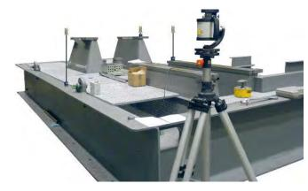
The **T330** creates a flat and level laser reference plane. We use the **R310** with its 80mm detector length to measure against this reference. The Software **ProLevel** lets you place these measurements on a template on site.
