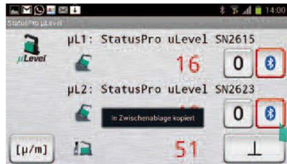
The μLevel will only transmit data to your Android when the μLevel is in the measurement mode I or II.
