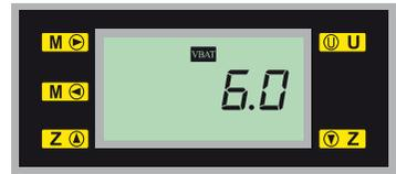
If the voltage is lower than 4 V, Low Voltage warning
