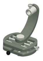
Using the swivel and tilt adapter you can align the laser level, irrespective of the surface below. The Adapter also allows for a parallel movement which is very useful when aligning the laser parallel to a reference object. The Adapter is accomodated with a 5/8" thread, and is also fitted with a three-point magnet arrangement underneath.
