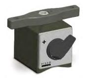
Block magnet (BT 943105) complete with a cross-bridge. This enables the mounting of a R545 Sensor or T250 laser with adapter BG 830780. Available attachment rods: BT 948155, BT 948156, BT 948157
