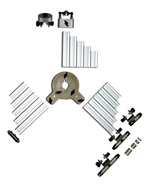
Borealign Kit 3 (BG 832080) is supplied with two different kinds of "feet" for Attachment C. They facilitate variable distances between the cams of the feet allowing measurement in bore-ways of differing depths.
