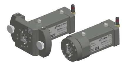
When you need to measure geometrical tasks, the R545 is a "hands down winner". Thanks to the symmetrical design of the housing, the R545 can be used for the most diverse of tasks! From linear guides, straightness of bore-ways, up to parallelism of printingmachine rolls or similar machines.
