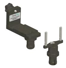
This adapter set is of great practical help for measuring flange parallelism. There is an adapter for the R545 Receiver and an adapter for the T330 Laser. After measuring the first flange, the adapters with their Sensors are exchanged, the tripods are remaining at their position. After re-aligning, the second flange can be measured parallel to the first.
