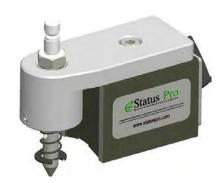
This adapter is used together with a R310. It separates the holding function from the measuring function. It is essential for flange measurement for example. The linear guide and the probe-tip contact rather than a surface contact is essential for precision measurements. Inside is a spring mounted that ensures a good contact to the object.
