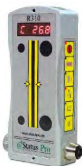
The R310 measures the position of the rotating laser beam. The CCD Sensor has total measurement range of 80mm. The beam forms an entire reference plane. The R310 is wireless and can measure up to a distance of 80m from the Laser.
