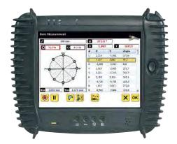
Rugged UMPC for industrial on-site. The UMPC offers protectors, shockproof design, holder for hand/arm.
