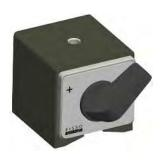
Block magnet for many measuring and fixing tasks. The upper surfaces has an M8 thread for attachment purposes. Dimensions:  $60 \times 50 \times 55$  mm, 750 N
